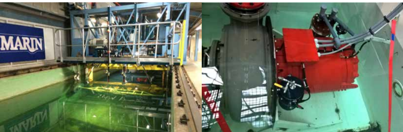
Figure 3 - above left: The pumping station model (submerged yellow model) mounted on the towing carriage of MARIN's concept basin (picture by MARIN). Above right: The open PM motor (courtesy IHC Mining).
