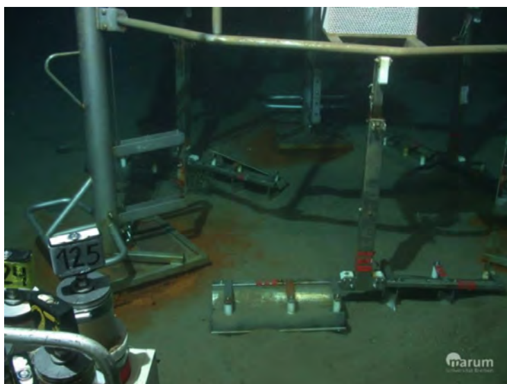
Above left: The Autonomous Sediment Disturber upon deployment at HAUSGARTEN off Svalbard. In the lower left corner push cores used for sampling by a remotely operated vehicle are visible. Image: MARUM at Bremen University and Thomas Soltwedel, AWI. Above right: The rotating plough-like unit disturbing sediments in a shallow water deployment to assess impacts on small sediment fauna and functions. Image: Thomas Soltwedel, AWI.
