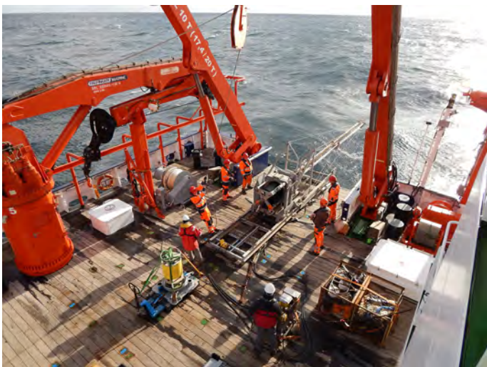
Left: Deployment of the piezometer from the RV Maria S. Merian
