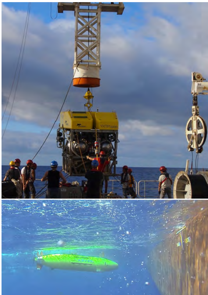
Figure 1, above left: The ROV VICTOR 6000 (top) and AUV ABYSS (bottom) used during the ODEMAR cruise aboard the French research vessel RV Pourquoi Pas? Figure 2, above right: Multibeam bathymetry map of the ODEMAR study area at the Mid Atlantic Ridge, showing the striated 13°20'N and 13°30'N detachments.
