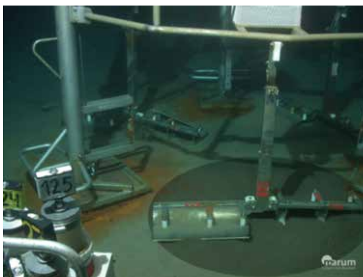
Figure 19 (above left): Two autonomous micro-profiler modules deployed during R/V SONNE expedition SO242/2 for benthic flux measurements at the 26 year old DISCOL disturbance tracks. Image: ROV KIEL 6000 Team / GEOMAR Kiel
