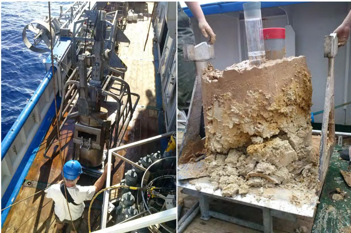
Figure 2: Left - Box-core on deck of RV Pelagia during the 2014 64PE388 MIDAS-TREASURE cruise in the Rainbow hydrothermal vent field area. Right - Retrieval of a box-core in the same cruise. A section of the first 1 m of the seabed is visible. Photos by A. Rabitti.
